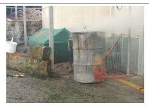
Figure 2: Fynbos fuel in smoke drum.
