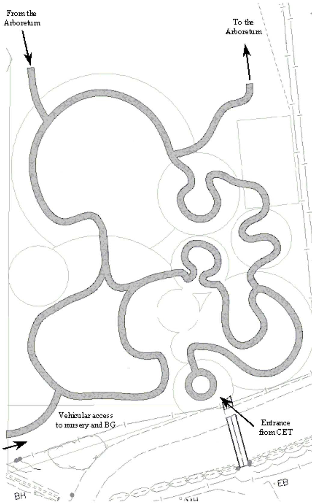
Figure 8.6 - Primary path around the site (at least 2-metres wide and capable of taking light horticultural vehicles)
